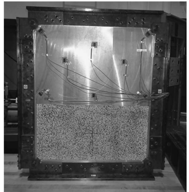
Fig. 4 Picture frame support mounted on a generic test panel.
